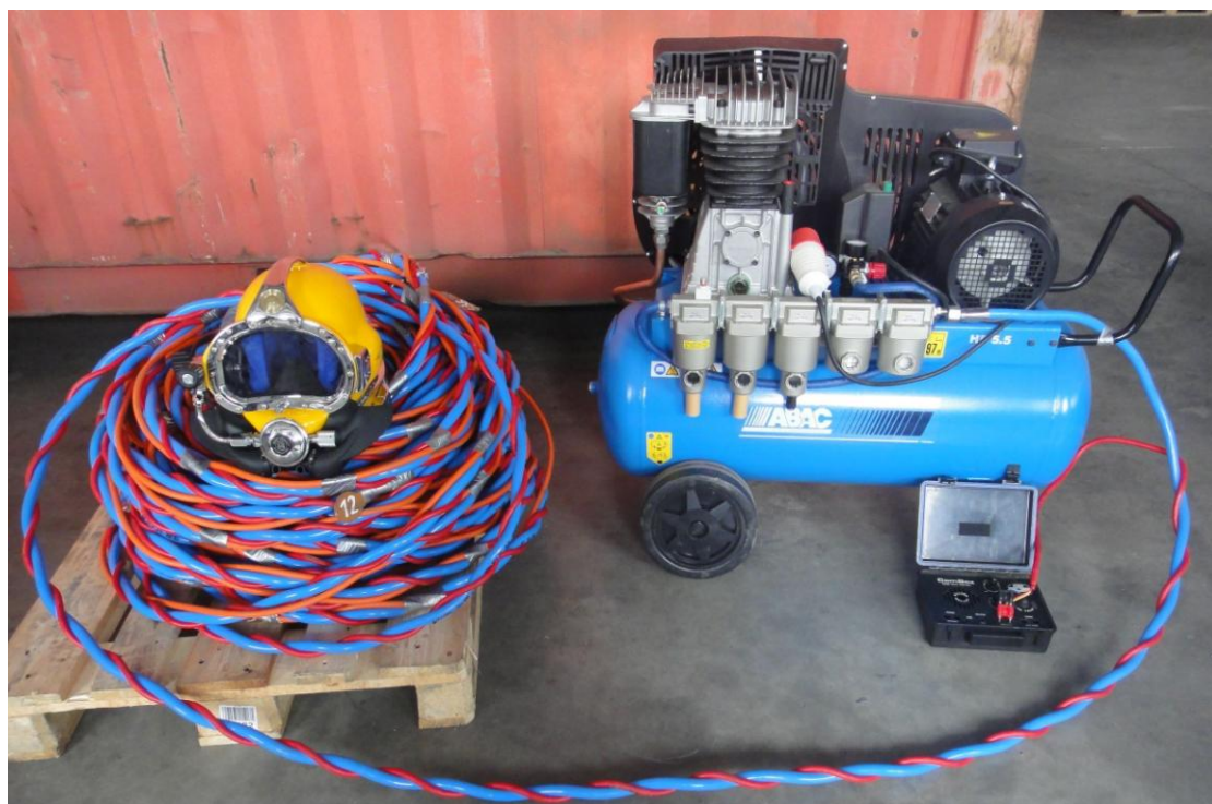
Pic. 3. MDC with MP compressor air supply
